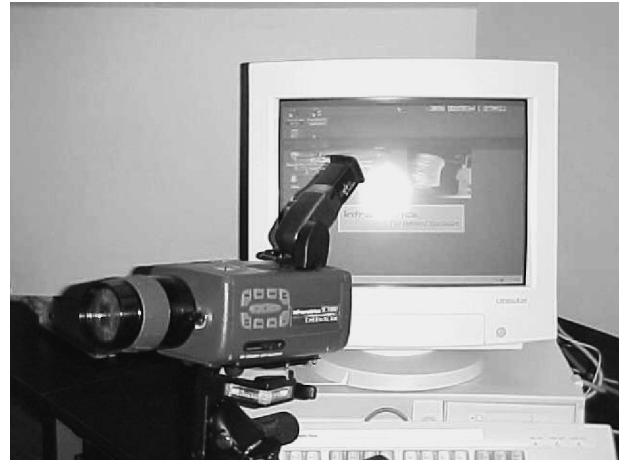
Fig. 1—Photograph of the infrared radiometric thermal imaging systems.
