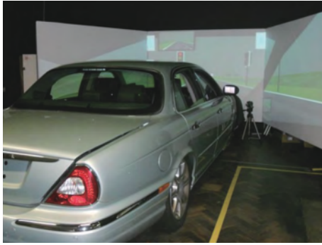
Fig. 1 Driving simulator with a virtual environment [47]
