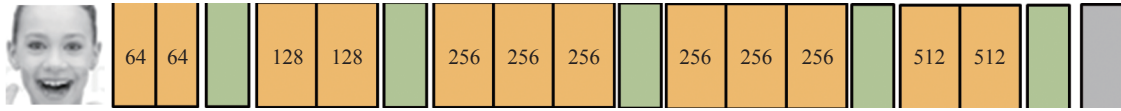
Fig. 1 Flowchart of our classification system. Yellow boxes, green boxes and grey boxes denote the 2D convolutional layers, max pooling layers and fully-connected layers, respectively. The number inside of the yellow box is the number of filters. And the number of neurons of the grey box is the same as the number of categories. Color versions of the figures in this paper are available online.
