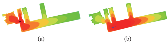
Fig. 7 The travel time map of the robot (a) and the target (b). The black circle represents the robot's current position. The blue circle with line denotes the target position and its predicted movement.
