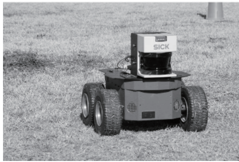
(a) Robot Pioneer 3-AT (P3-AT) used for experiment
