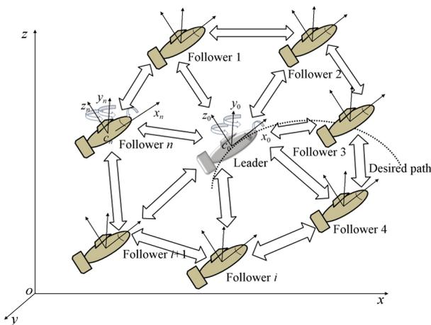
Fig. 1 Schematic representation of cooperative control of AUVs (leader-follower approach)
