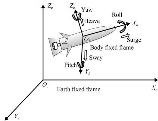
Fig. 3 Schematic representation of an AUV showing forces and torques
