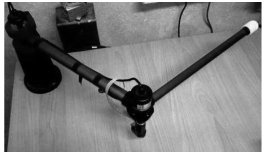
Fig.1 The two link planar manipulator employed for experimental results
