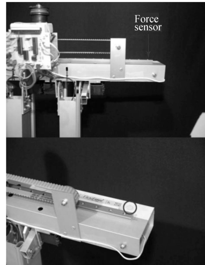
Fig. 20 Force sensor at the edge of the hip to measure the magnitude of the external disturbance
