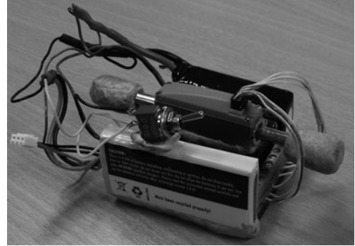
Fig. 2 Self-contained capsubot system
