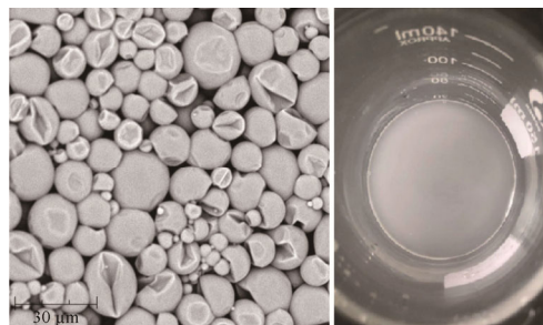
Fig. 1 Appearance of the MEPCM and its suspension [41]
