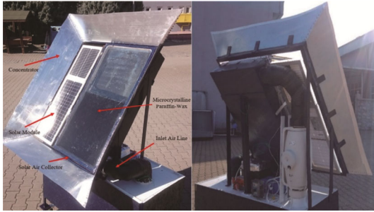
Fig. 3 Manufactured concentrated solar air collector with a heat storage unit
