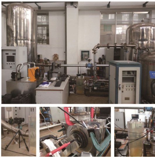
(a) High-speed photography (b) Installation of model pump (c) Water tank
