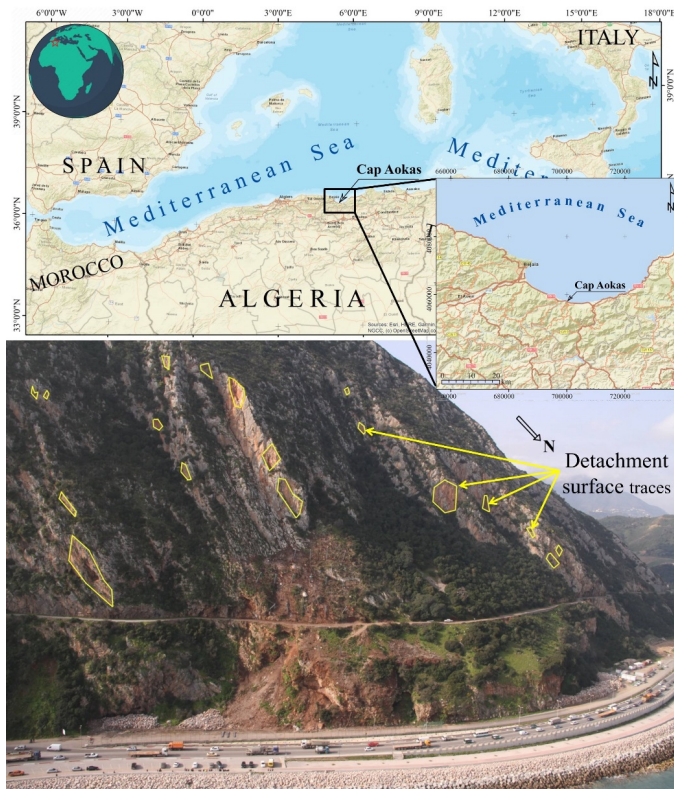
Fig. 7 Geographic position of Cap Aokas cliff, and photograph of detached blocks located on N130° oriented.
