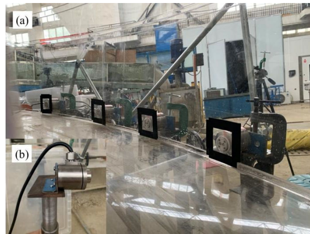
Fig. 4 Schematic diagram of sensor installation: (a) sensors installed at the bottom of the concave bank (b) sensor bracket.
