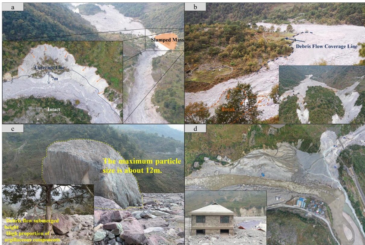
Fig. 5 a) Field observation of the landscape in the corner (propagation area A), which indicates that the speed of the passing debris flow was relatively slow; b) the debris flow overrunning phenomenon occurred in the accumulated & restarted area; c) the largest particle size (approximately 12 m in diameter) found in the area accumulated & restarted area; d) aerial view of the debris deposits at the gully entrance and the nearby buried house.
