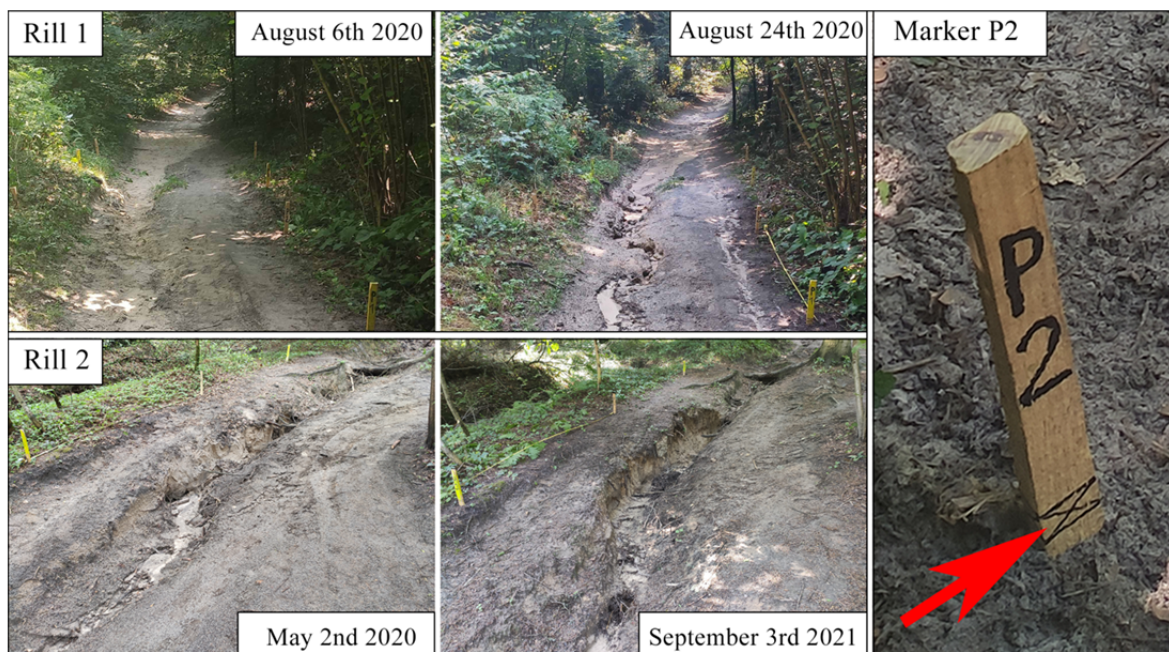
Fig. 2 First and second rill during SfM scanning, Marker P2 as an example of one of the eight GCPs placed on each test plot, arrow points to painted target.
