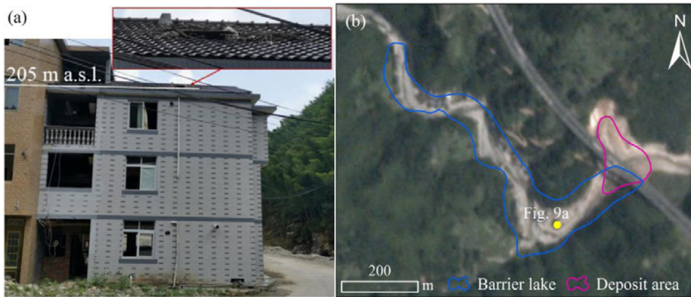
Fig. 9 (a) The floating weeds and debris on the roof of a three-story building and (b) The barrier lake caused by the Shanzao landslide. The base map is from a plant image with a 3 m resolution.
