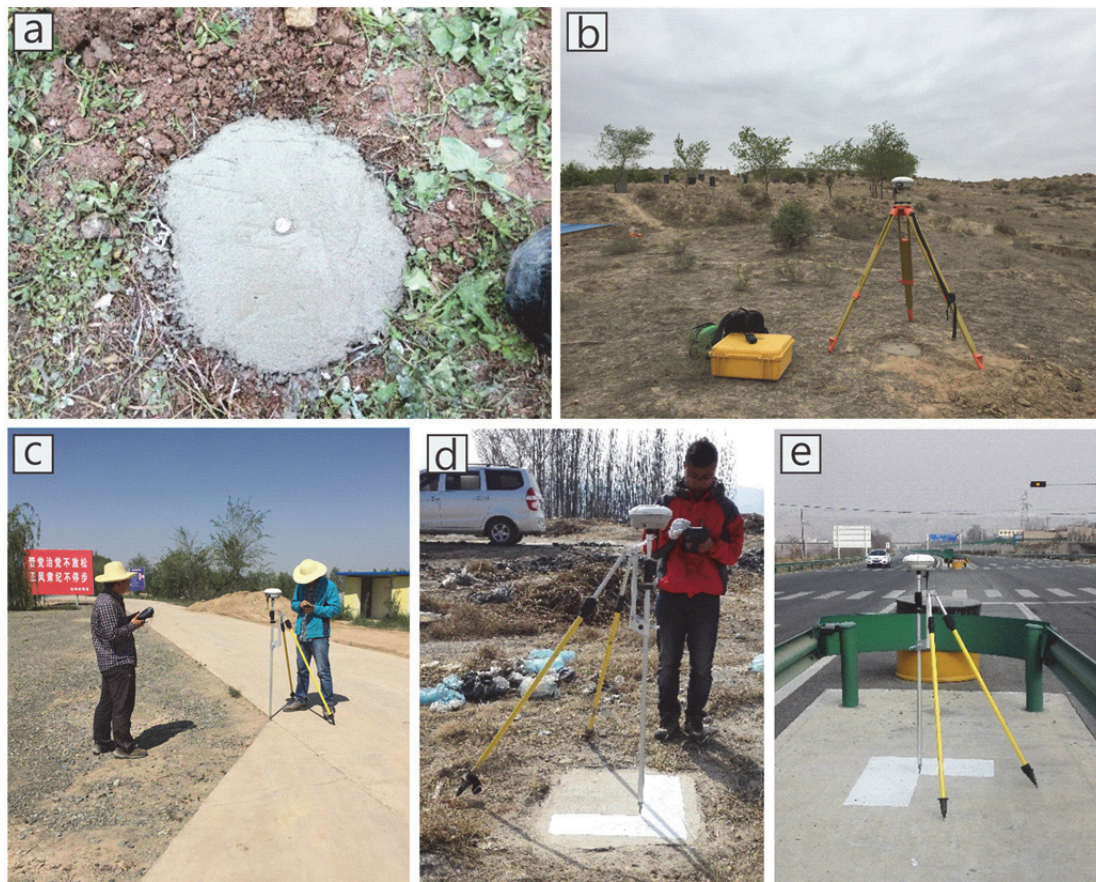
Figure 3 Ground control points (GCPs) targets and their measurement by the differential global positioning systems (DGPS). (a) permanent GCP; (b) static GPS measurement; (c) natural GCP; (d) artificial GCP; (e) GCP on the road.
