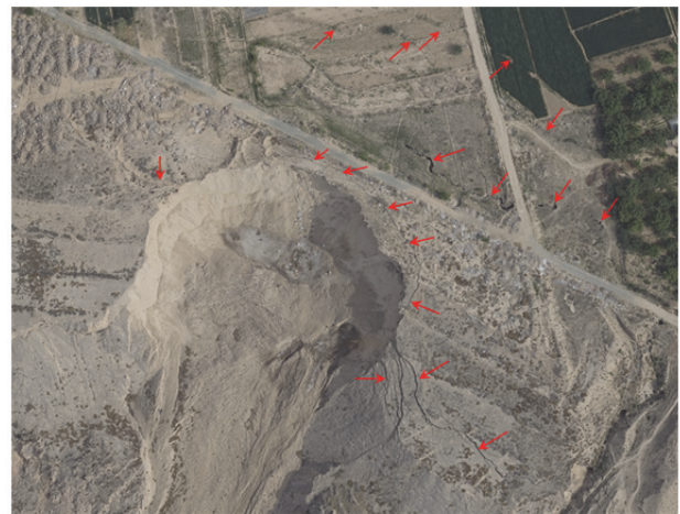
Figure 9 The orthophoto of the DC#3 landslide taken in May 2016. The red arrow indicates the position of cracks and sinkholes around the DC#3 landslide.
