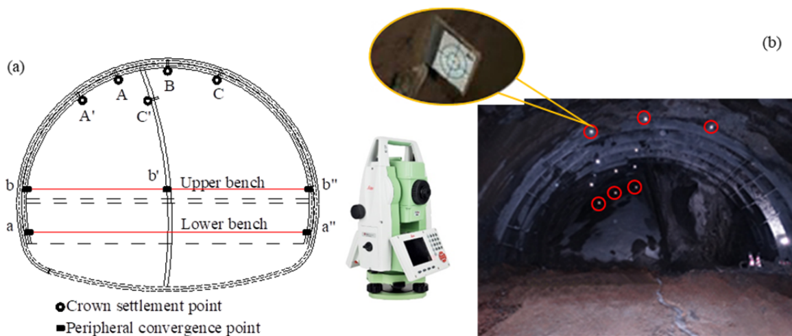
Figure 5 Layout of measuring points of tunnel deformation; (a) Layout of measuring points in transverse section. (b) In-site measuring points.
