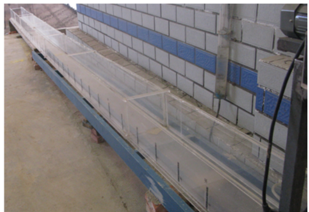
Figure 5 Experimental sediment flume with varying bed slopes of upstream and downstream.
