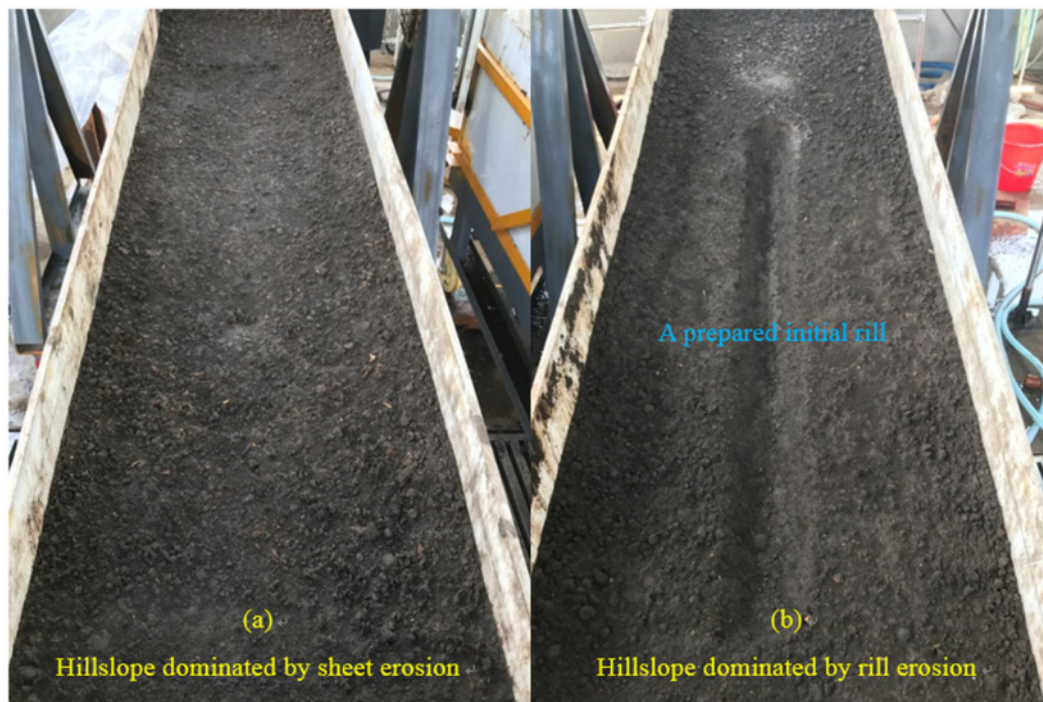
Figure 1 Test soil pan with hillslopes dominated by sheet erosion (a) and rill erosion (b).
