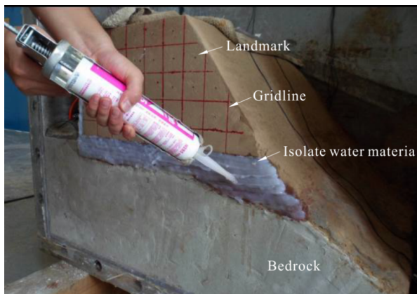
Figure 6 Model preparation (grid lines, landmarks and isolate water material).
