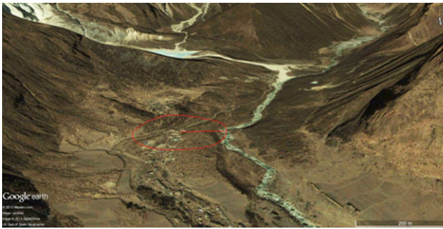
Figure 18 Satellite image of the Samagaun settlement and adjacent Buri Gandaki River (ca. 28^{\circ}35'24.69'' N, 84^{\circ}38'29.93'' E) at 3542 m a.s.l. The red line that starts at the riverside and ends at the centre of the circle represents the distance between the Samagaun settlement and the Buri Gandaki River, i.e., approximately 165 m. The approximately 80-m-high river-right Birendra Kund lateral moraine forms a natural dam. This glacial landform protects the adjacent valley, including Samagaun village, from splash waves generated in the lake. Therefore, the potential flood waves cannot flow southeastward, and the flow must follow the course of the river.
