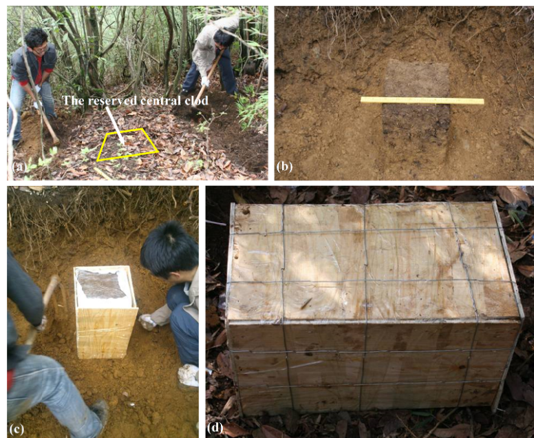
Figure 3 The sampling procedure for each undisturbed soil core. (a) a pit was dug and the central clod was reserved; (b) four vertical lateral sides and the top surface of the soil column were well prepared, the length of rule is 50 cm; (c) the soil column was wrapped with plastic film, cloth and wooden blocks; (d) soil column was tighten with iron wire.
