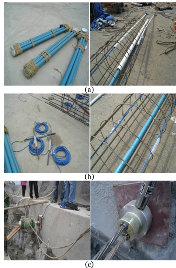
Figure 6 Field monitoring instruments. (a) inclinometer; (b) strain gauge; (c) anchor strain gauge.
