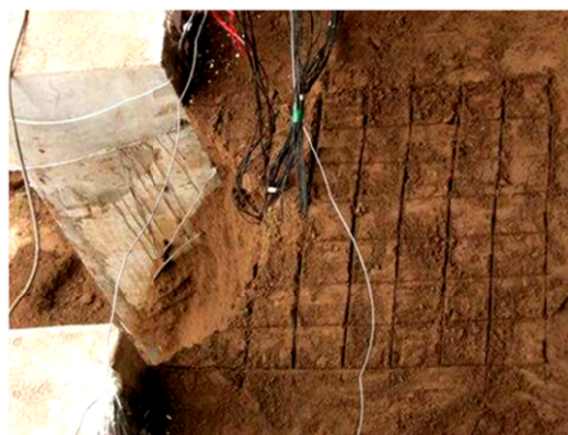
Figure 3 Instability phenomenon of soils between cantilever piles in tests.
