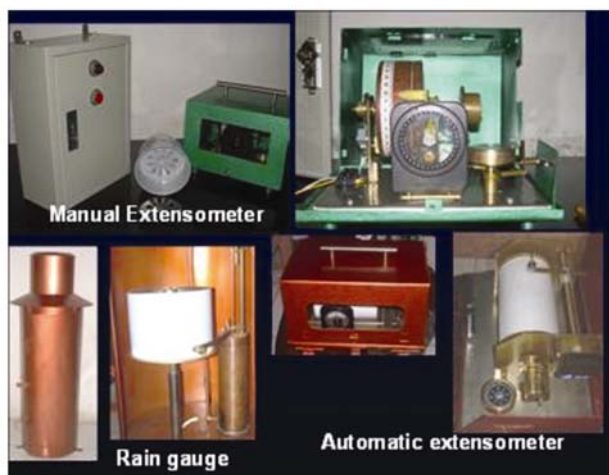
Figure 7 Early warning system equipments consisting of a) manual extensometer with the control panel and siren and b) rain gauge, developed by Fathani et al. in 2008.
