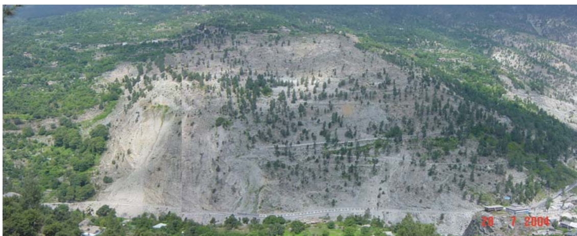
Figure 8 View of the Pawari landslide in 2005. It is a complex landslide involving different movements in different parts of the landslide. The landslide greatly increases the width from 500 m to 1200 m during 1990 ~ 2005.
