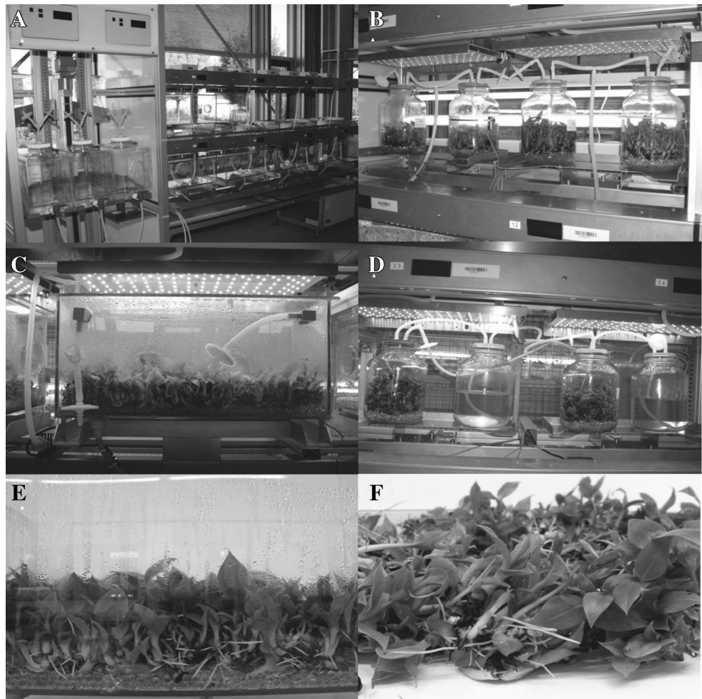
Figure 1. Micropropagation of banana ( Musa spp. cv. 'Grande naine, AAA) in temporary immersion systems. (A) New type of TIS (type 2) with lighting from the top and medium change by gravity. (B) Five-liter TIS (type 1) with lighting from the side (white fluorescent lamp). (C) Polycarbonate box (PC) from new type of TIS (type 2) illuminated by LEDs with banana shoots after 4-wk growth. (D) Five-liter TIS standard lightened LEDs with banana shoots after 4-wk growth. (E) Aspect of banana plants in plastic box from new type of TIS (type 2) after 7-wk culture. (F) Aspect of banana plants harvested from standard TIS with white fluorescent light from the side and additional gassing at 7-wk culture.
