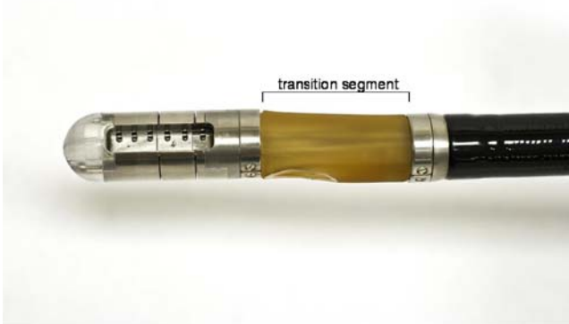
Figure 3 Capsule with flexible transition that allows introduction through the oro- and hypopharynx.
