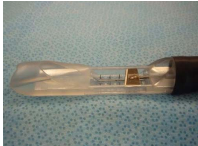
Figure 9 The 5-cm long rigid excision capsule with vertical anchor needles, suction ports, guillotine excision blade, and a longitudinal injection needle.
