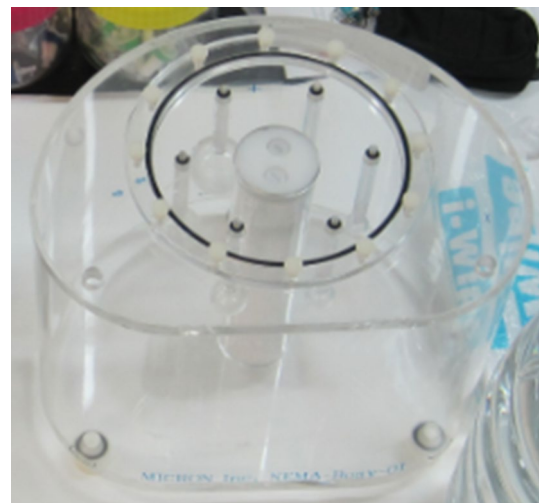
Fig. 1 This was the phantom used for standardization, which had six hot spheres (10, 13, 17, 22, 28 and 37 mm)
