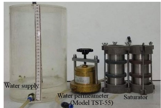
Fig. 5 The setup of the falling head permeability test
