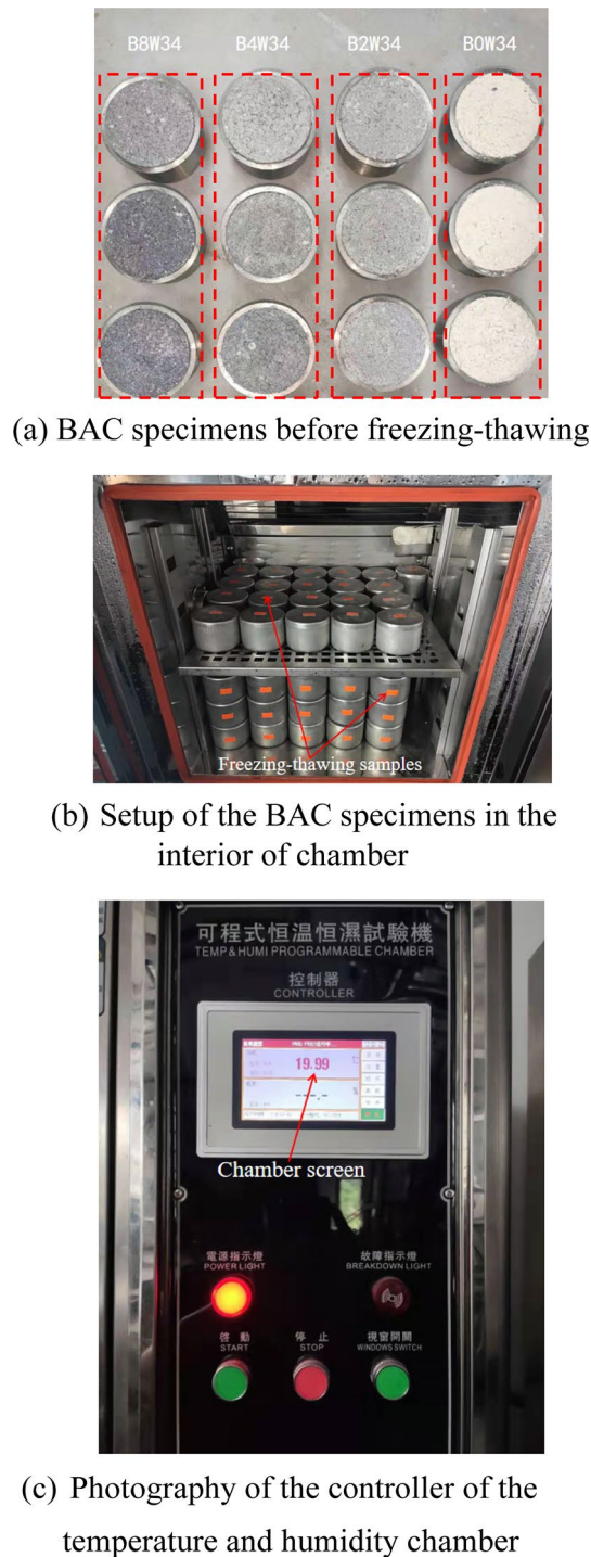
Fig. 4 Arrangement of the BAC specimens in the temperature and humidity control chamber
