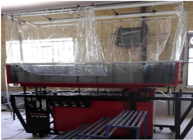
Fig. 3 Physical soil model and rainfall simulator used in laboratory tests
