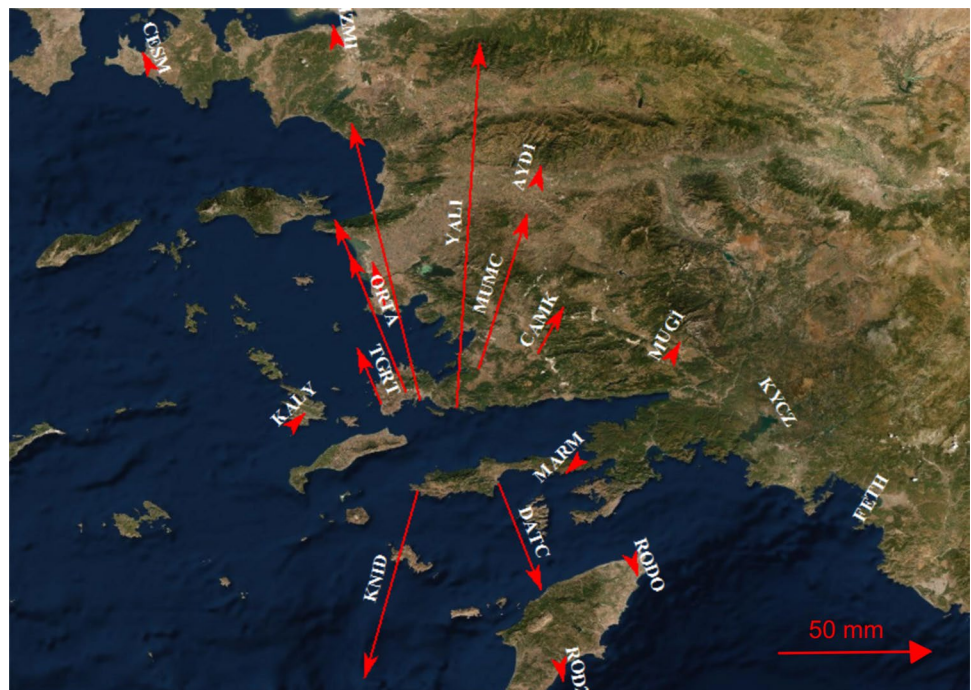
Fig. 7 Coseismic displacements, recorded by GPS/GNSS stations (modified from Tiryakioğlu et al. 2018)
