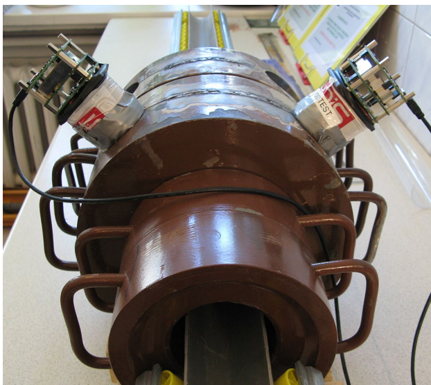
Fig. 2 Gamma logger spectrometer GLGT adapted to low-radioactive core measurements. Two independent BGO detectors were placed at a 90° in lead tunnel shielding
