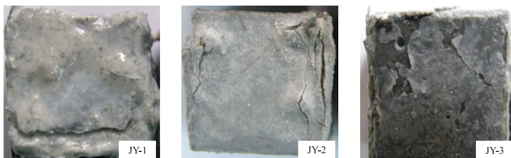
Fig.2 View of paste samples immersed in 5% MgSO_4 at 6 °C for 240 days
