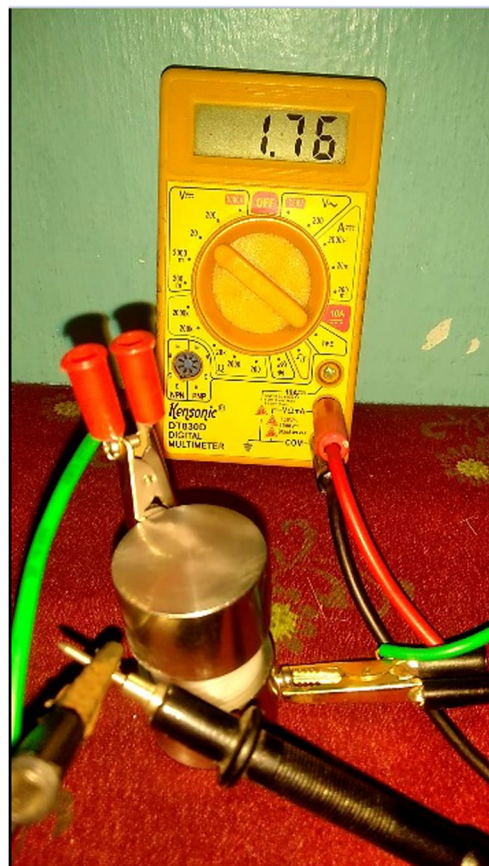
Fig. 15 Open Circuit Voltage for 30 NaAlg: 70 \text{NH}_4\text{ClO}_4
