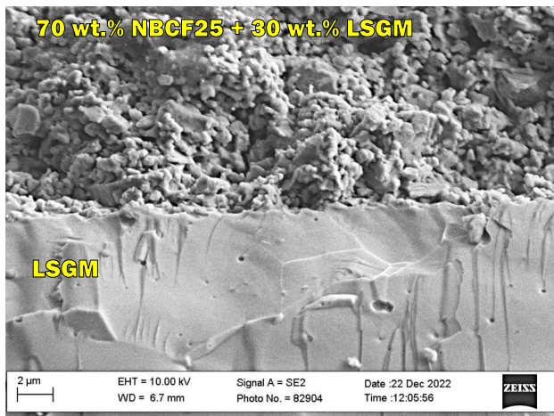
Fig. 6 Cross-sectional SEM images of \text{Nd}_{0.75}\text{Ba}_{0.25}\text{Co}_{0.8}\text{Fe}_{0.2}\text{O}_{3-\delta} (NBCF25)/ \text{La}_{0.8}\text{Sr}_{0.2}\text{Ga}_{0.8}\text{Mg}_{0.2}\text{O}_{3-\delta} (LSGM) composite cathode screen printed onto LSGM electrolyte
