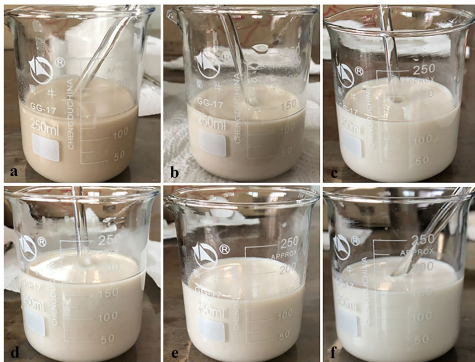
Fig. 1 The suspensions after hydrothermal synthesis with various molar ratios of Li/M/P: a 1:1:1.0, b 1:1:1.2, c 1:1:1.4, d 1:1:1.6, e 1:1:1.8, and f 1:1:2.0
