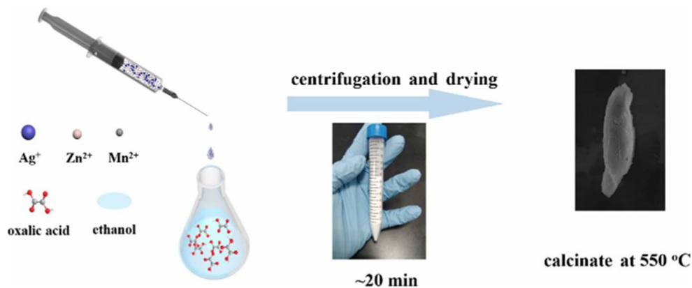
Fig. 1 The schematic illustration of the preparation process of Ag/ZMO composites
