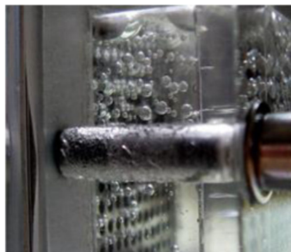
Fig. 8 Photograph of the carbon dioxide bubble coming out from the openings of ACC in a passive DMFC [92]
