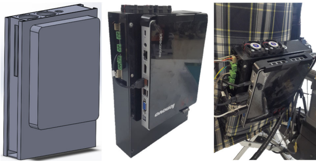
Fig. 13 Main control unit; composed of a computer (mini PC), a microcontroller unit and a power management unit
