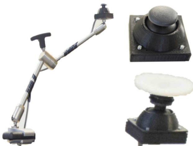
Fig. 8 Hand and chin input modules; hand (top right) and chin (left below) joysticks were mounted on a three degree of freedom (DOF) actuator installed on the wheelchair. The 3 DOF actuator could be used to adjust the joystick position individually for each user
