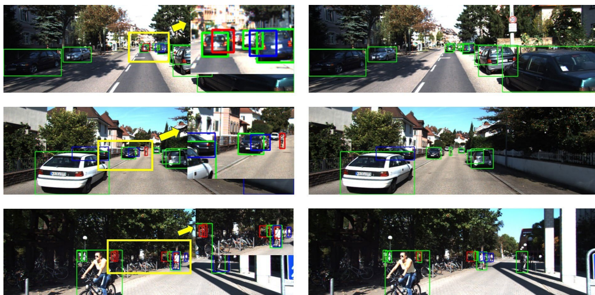
Fig. 8 Visualization of detection results of YOLOv8-n detector (left) and DF-YOLO detector (right) based on the KITTI dataset. Green, blue, and red boxes represent true positives (TP), false positives (FP), and false negatives (FN), respectively. Yellow boxes indicate zoomed-in views
