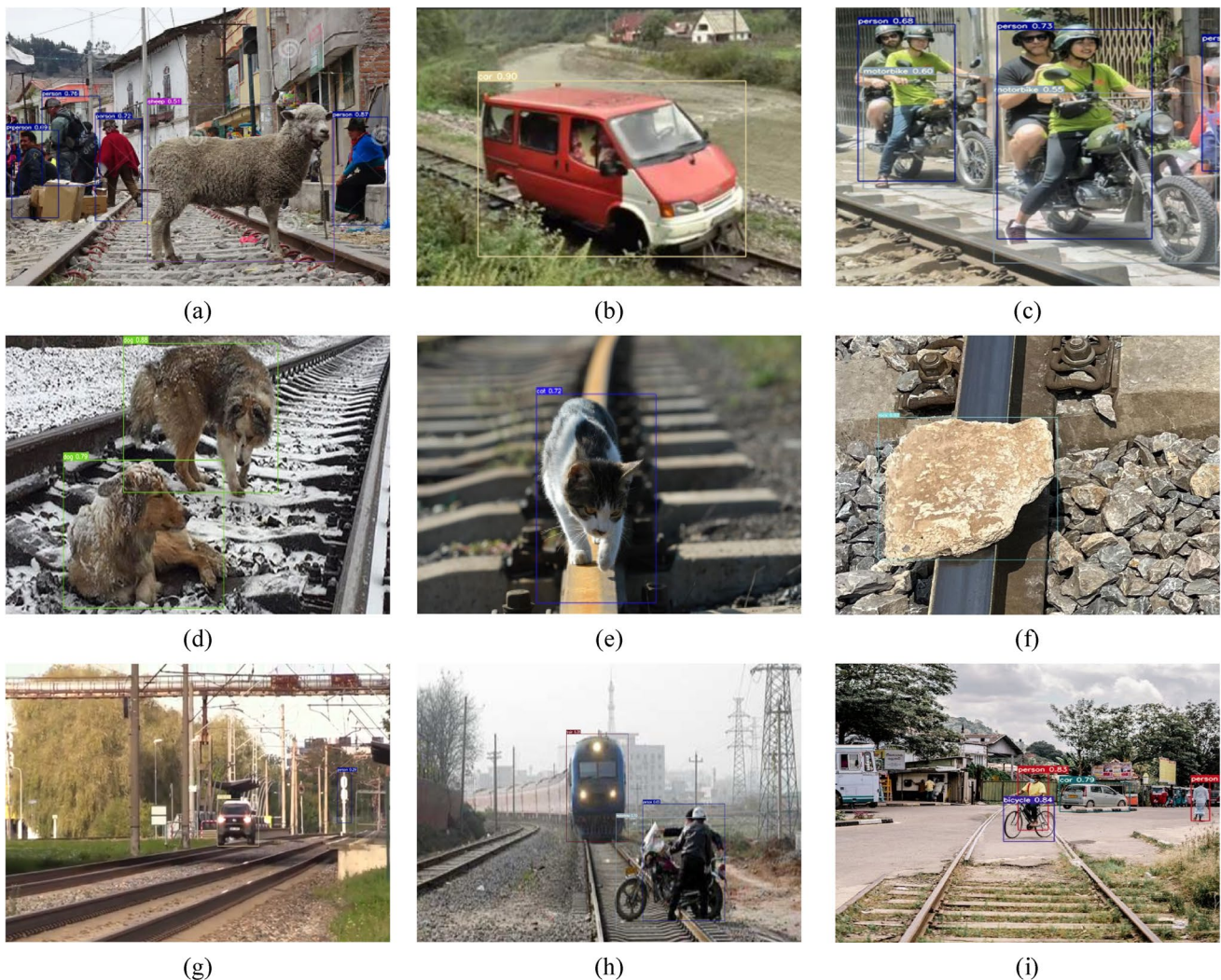
Fig. 13 Recognition results of foreign bodies in railway tracks
