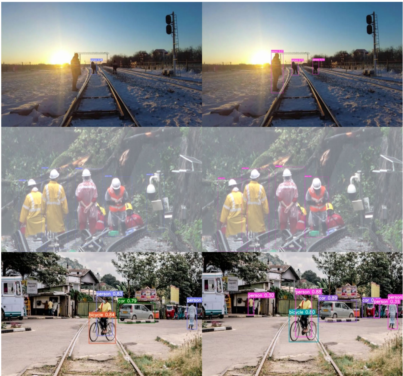
Fig. 12 Example of railway foreign object intrusion detection results
