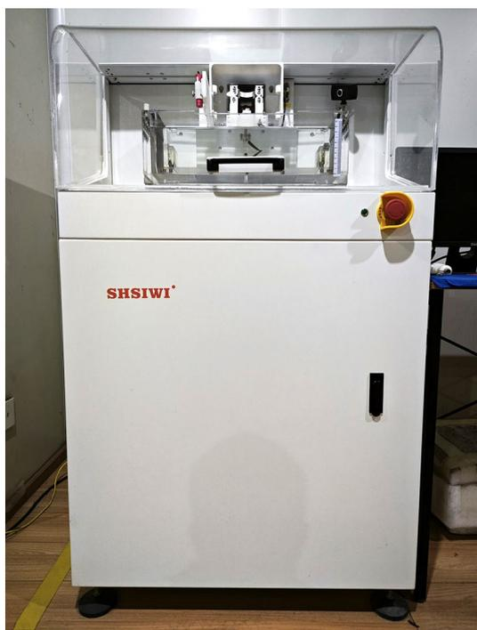
**Fig. 5** The SAM tool for scanning and collecting ultrasonic images of PEC
