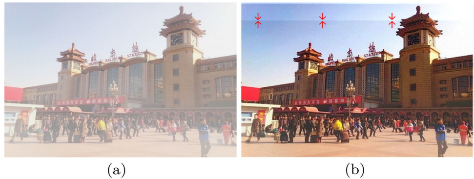
Fig. 6 Dehazed image appears dividing line. a is the original, b is the dehazed image
