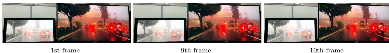
Fig. 13 Dehazing results on dash cam video. The left display is before defogging, the right is after defogging
