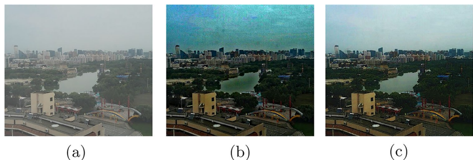
Fig. 9 The comparison of the dehazing effect with using DCP only and DCP with adaptive threshold segmentation. a Is the original image, b uses DCP only, c uses DCP with adaptive threshold segmentation
