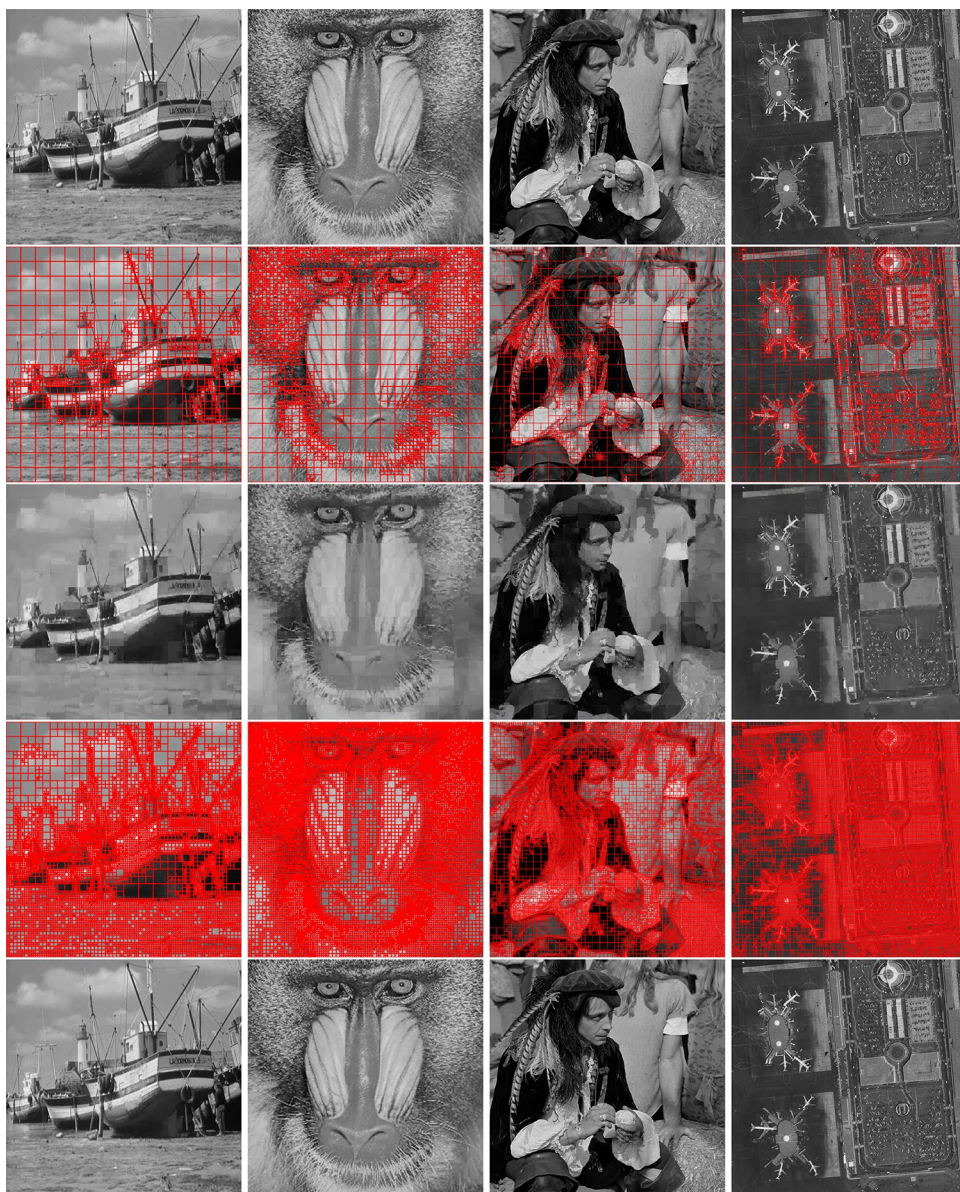
Fig. 1 Fractal image compression with quadtree partition using large images. Original images (first row). Resultant quadtree partitions and decompressed images with \tau_{01} = 20 (second and third rows). Resultant quadtree partitions and decompressed images with \tau_{01} = 5 (fourth and fifth rows)
