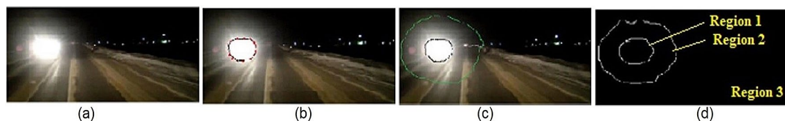
Fig. 3 Process of segmentation of a frame with high beam and glare. a The original frame b core headlight portion (Region 1) is extracted c Glare portion (region 2) is extracted d three regions (1, 2, and 3) are segmented
