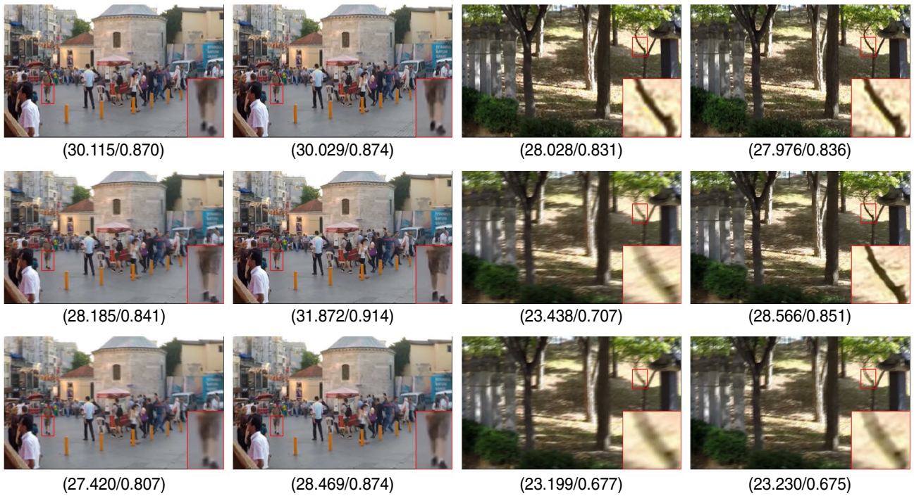
Fig. 5 Performance test of motion deblurring sub-CNN: the first and third columns are the input images, and the second and fourth ones are the SR outputs; from top row to bottom one are LR images,
