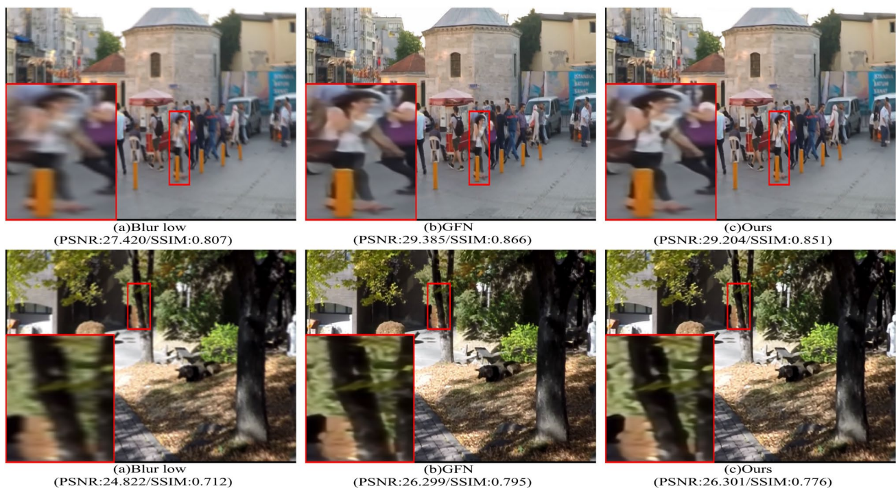
Fig. 8 Visual comparisons to some state-of-the-art methods: a the input blur and LR images (from GOPRO dataset [15]); b GFN (gated fusion network) of Zhang et al. [36]; c our proposed approach
