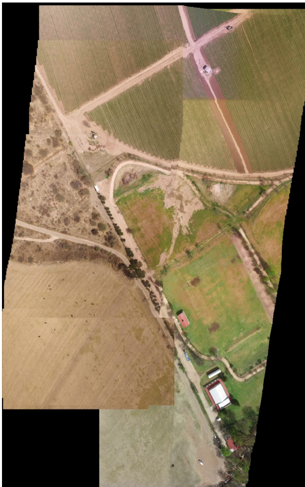
Fig. 1 Aerial mosaic performed on a 100 m high flight, using hash table in a GPU architecture. The distance travelled by the drone for the generation of the mosaic was 1.7 km. A video of this work for reviewing purposes is found at https://youtu.be/CRT3v1n6xtQ
